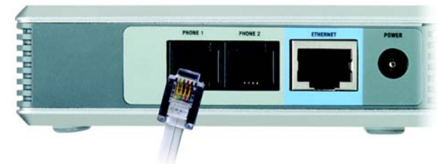
Figure 3-2: Connect the RJ-11 Telephone Cable
