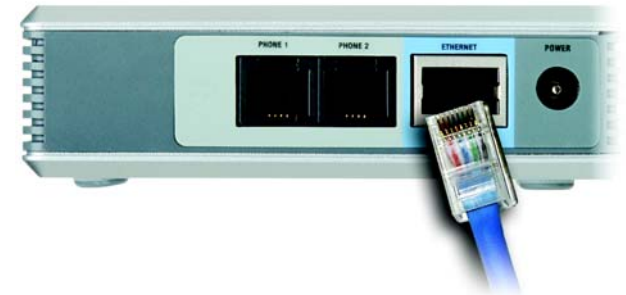
Figure 3-3: Connect the Ethernet Network Cable
