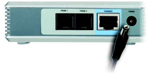
Figure 3-4: Connect the Power
